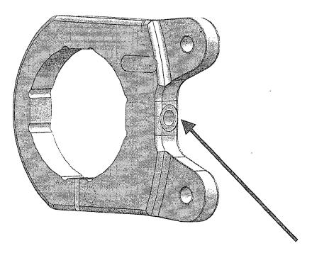
This hole is not drilled completely through on some brackets for a reason. the last small amount of the hole that isn't threaded is used as a pilot to drill through the tube with a 21/64 drill. Once the holes drill through the tube, run a 3/8-24 tap through the hole and through the tube. Once that is complete, insert the bolt.
